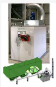
Aggthem Aggregate Heating Systems for sand & gravel bins enable plants to produce concrete at sub-zero temperatures. In contrast to saturated steam-based systems, the hot-dry air (248°F/120°C) Aggtherm equipment uses as a heating medium does not impact the water/cement ratio in the concrete mixture. An additional option for preheating mix water equips operators with additional mixture temperature control.
