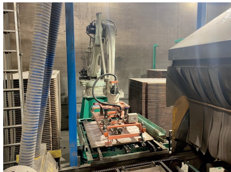
Many concrete production facilities utilize steel pallets, and because all the pallets are almost always one size, shape, and weight, a robot pallet accumulator was right for the job.
