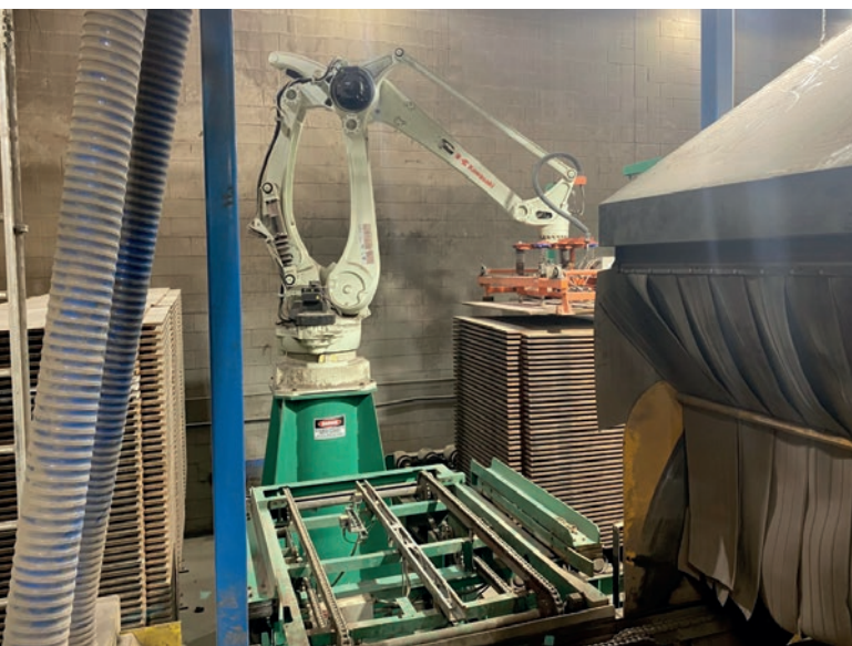
Many concrete production facilities utilize steel pallets, and because all the pallets are almost always one size, shape, and weight, a robot pallet accumulator was right for the job.
