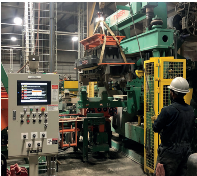
Midwest crew completing a quick mold change on their Model S
