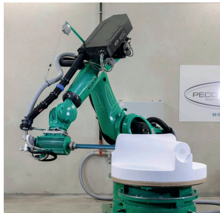
Fig. 6: Onto the arm of the robot a tool is fixed for milling to millimeter precision the workpiece made of Sagex (expanded polystyrene foam), wood or other plastics for producing the negative forms. Tool change is fully automatic.
