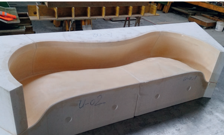
Figs. 8a+b: Part of formwork made of polyurethane foam for a fountain in the English garden in Interlaken ...
