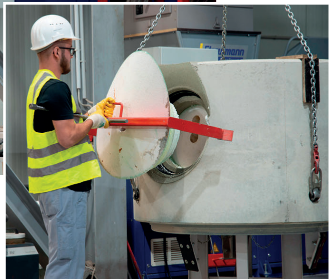
Fig. 7: The negative channels and the blockout bodies, like here for the pipe connections, can be easily removed during demolding.
