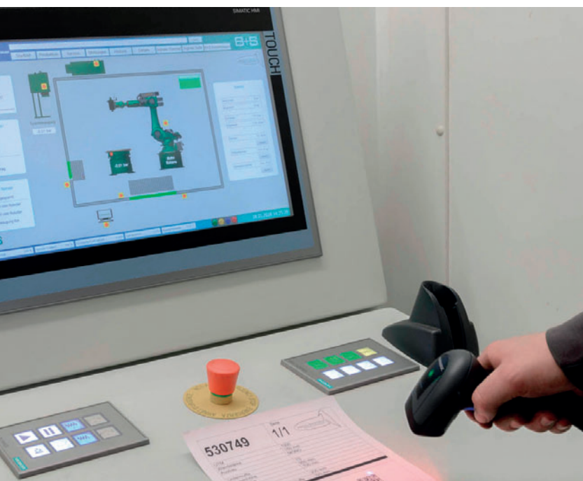
Fig. 5: The operator at the control desk scans the job order with QR code generated and printed out by the manhole configurator with a handheld scanner and in this way passes on the required production data to the control of the processing station of the B+S Peco-system.
