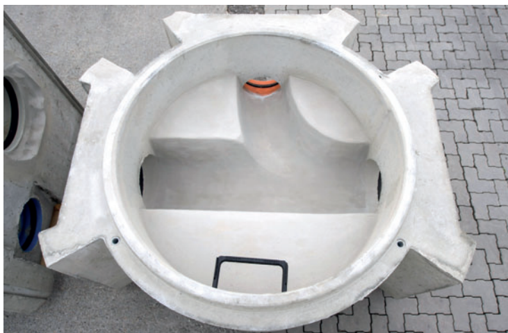
Fig. 2b: The completed manhole base with the specified drainage channel, the counterpart of the negative form made of polystyrene (compare Fig. 2a)
