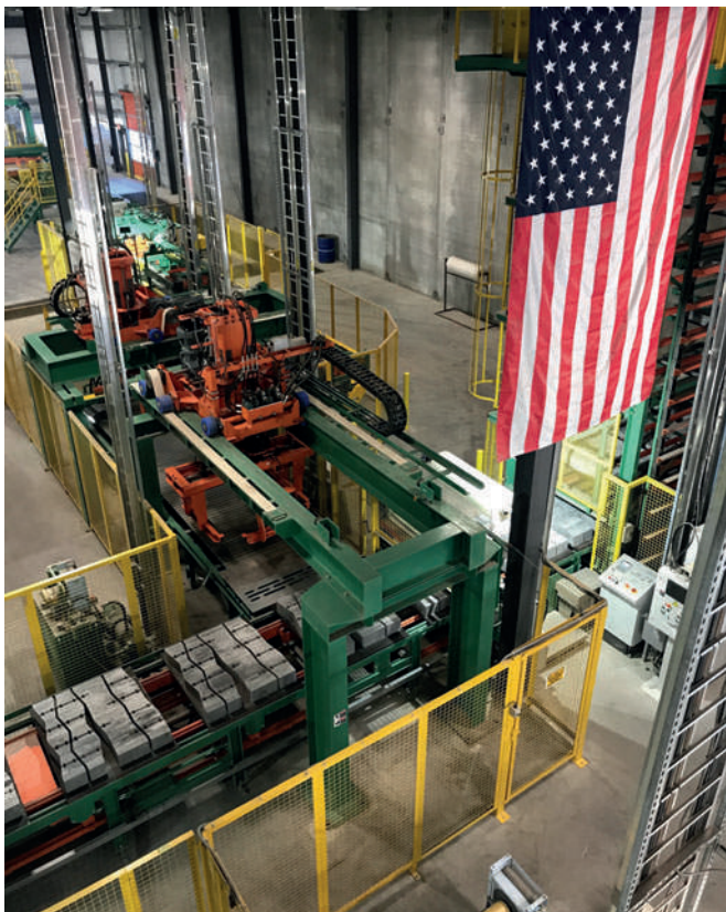
It was decided to install two types of Cubers available from Pathfinder/Tiger Machine, the CC-Cuber and the CP-Cuber.
