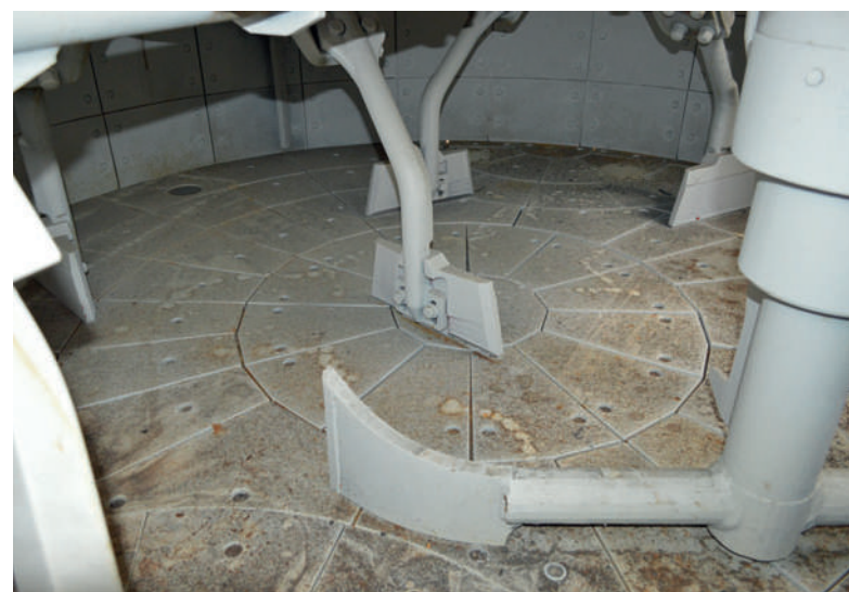
The THT series incorporates the patented mixing turbine arm
