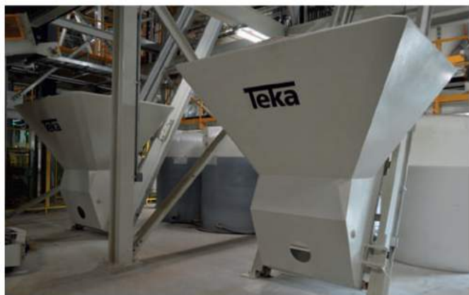
THT mixers have Variable Frequency Drives (VFD's) as standard equipment
