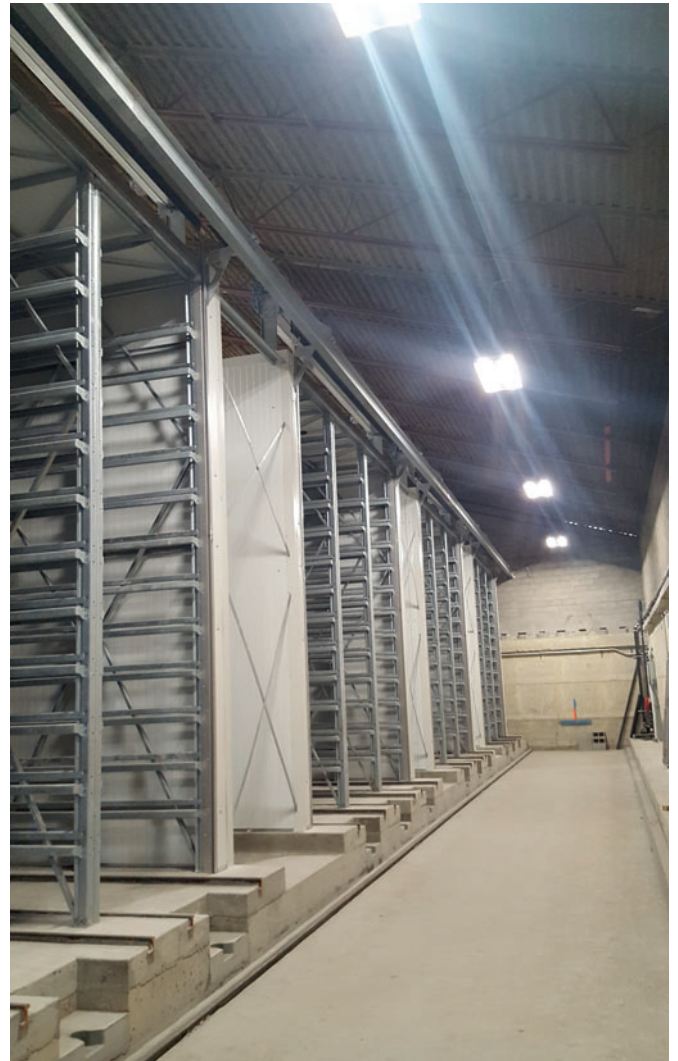
CureTec was selected to provide an insulated, galvanized rack system and the curing system.
